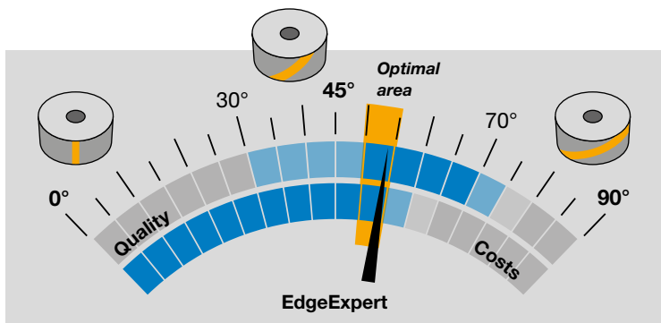
Leitz EdgeExpert: optimally adjusted shear angle
