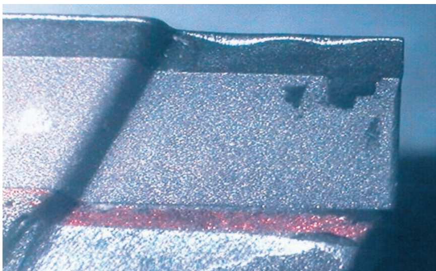
Snijkant afronding na inzet in GFK.
